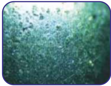
Pitting corrosion on balls of deep groove ball bearing
