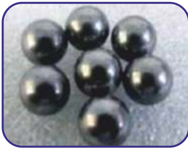
Pitting corrosion on balls of deep groove ball bearing
