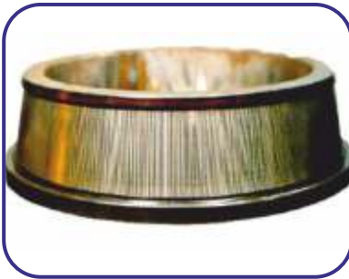
Craters formed by current leakage resulting in fluting
