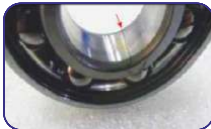
Forced fracture due to excessive interference fit
