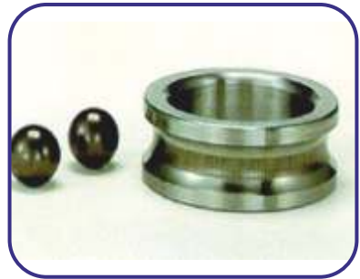
Fluting on inner ring raceway with dark colored balls
