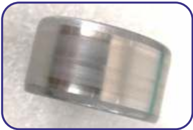
Wear and indentation on inner ring raceway of Cylindrical Roller Bearing due to soft foreign particle contamination
