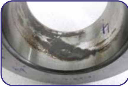
Moisture corrosion on Inner race bore of Taper Roller Bearing
