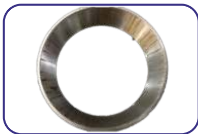
Brinelling mark on cup raceway due to vibrations
