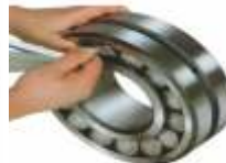
Checking clearance with feeler gauge
