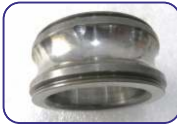
True brinelling mark on inner race shoulder of Ball Bearing due to improper mounting/dismounting
