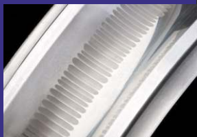
Electrical fluting damage
