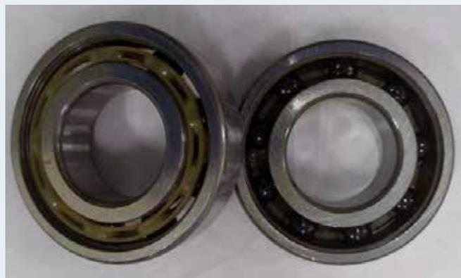
6206 bearing with MoS2 coated bearing balls
