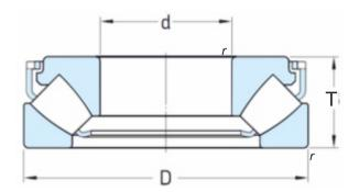
Equivalent bearing load dynamic Pa = Fa +1.2F
