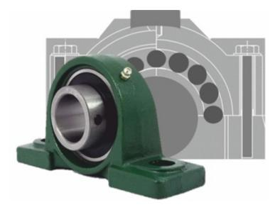
NBC offers Pillow blocks for both standard and special applications. The Pillow blocks are made of cast steel housing and meet the harsh environmental conditions of industry. The units are with strong base and have radial insert ball bearing with grub screws. Sealing protect from dirt and dust.
