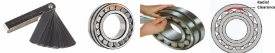
Checking clearance with feeler gauge
