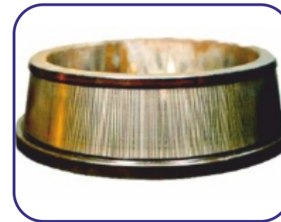
Craters formed by current leakage resulting in fluting
