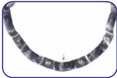
Excessive wear of cage pocket as a result of flaking on single ball
