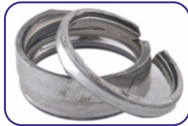
Fatigue fracture of an outer ring from snap ring groove in Double Row Angular Contact Ball Bearing caused by axial loading
