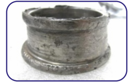
Inner ring of taper roller bearing plastically deformed and discolored due to lack of lubrication or loss of lubricating properties in high temperature application
