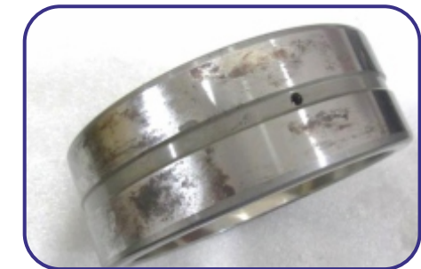
Moisture corrosion on outer ring of Spherical Roller Bearing
