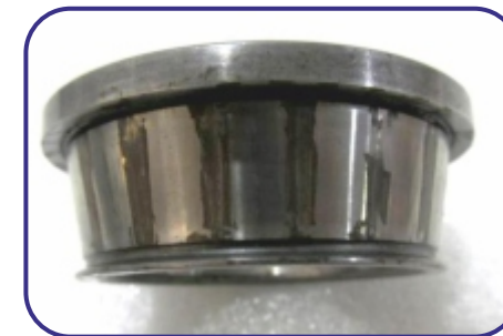
Contact corrosion on cone raceway of Taper Roller Bearing at roller pitch distance
