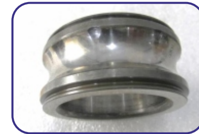
True brinelling mark on inner race shoulder of Ball Bearing due to improper mounting/dismounting
