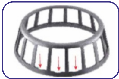
Heavy wear on retainer pockets of taper roller bearing due to over rolling of hard contaminants between rollers head surface and retainer pockets
