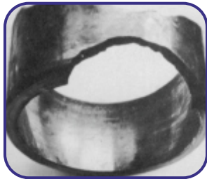
Fatigue fracture of Outer ring caused by insufficient support in the housing
