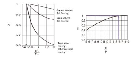
From both graphs f1, f2 are equal to 1 for the condition C/P= 16 and Fa= 0.2 Fr. For other condition like C/P and Fa= 0.2 Fr, corresponding values of  $f_1$ ,  $f_2$  to be multiplied for correcting the limiting speed.
