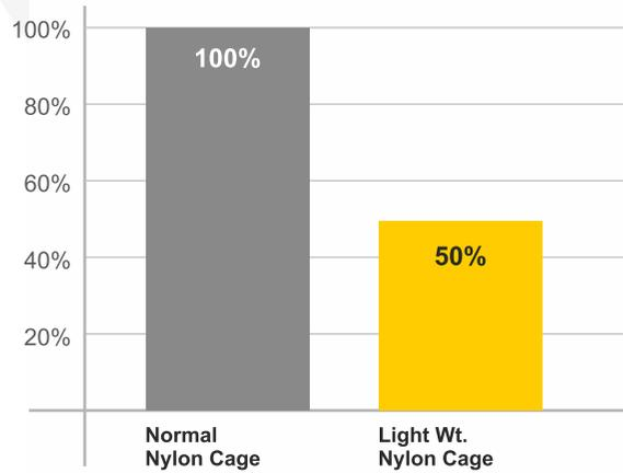
Cage Deflection at 20000 rpm reduced by 50% of conventional cage
