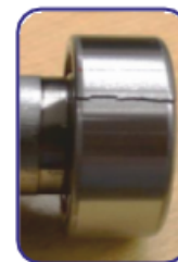
Forced fracture of Outer ring caused by a direct impact blow
