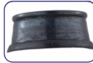
Inner ring of taper roller bearing plastically deformed and discolored due to lack of lubrication or loss of lubricating properties in high temperature application
