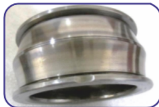
Wear and indentation on inner ring raceway of Double Row Spherical Roller Bearing due to soft foreign particle contamination
