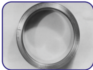
Thermal cracking on cone bore of taper roller bearing
