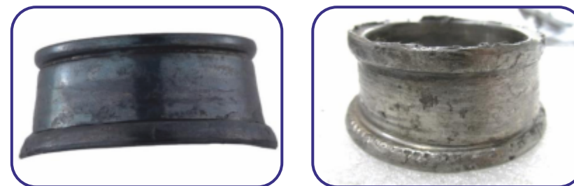
Inner ring of taper roller bearing plastically deformed and discolored due to lack of lubrication or loss of lubricating properties in high temperature application
